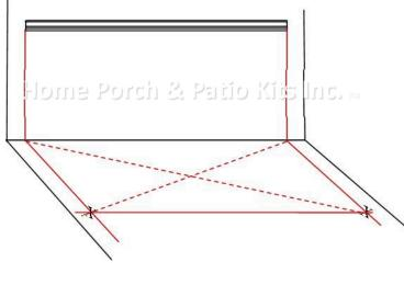
a windy day!). "Square" up the awning perimeter by temporarily installing an awning pan about every 6 to 10 feet. . This is IMPORTÁNT!
